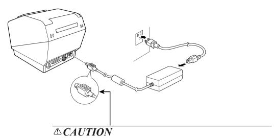
When disconnecting the cable, take hold of the cable connector to pull it out. Releasing the lock makes it easy to disconnect the connector.
